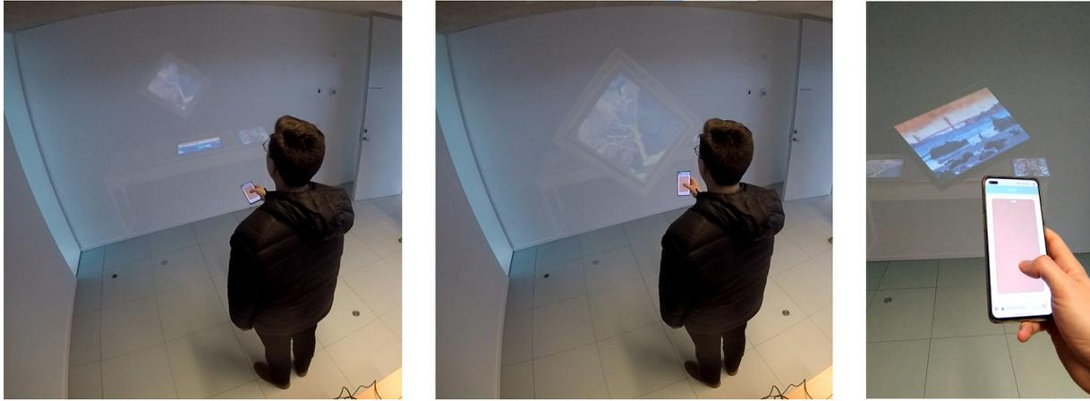
**Figure 6** *In the 3D setup, the participant uses a smartphone to control a cursor on the screen. It can be used to pick up, move, and tilt the virtual paintings. The first two images are video stills from the experiment. The third is a staged closeup.*
