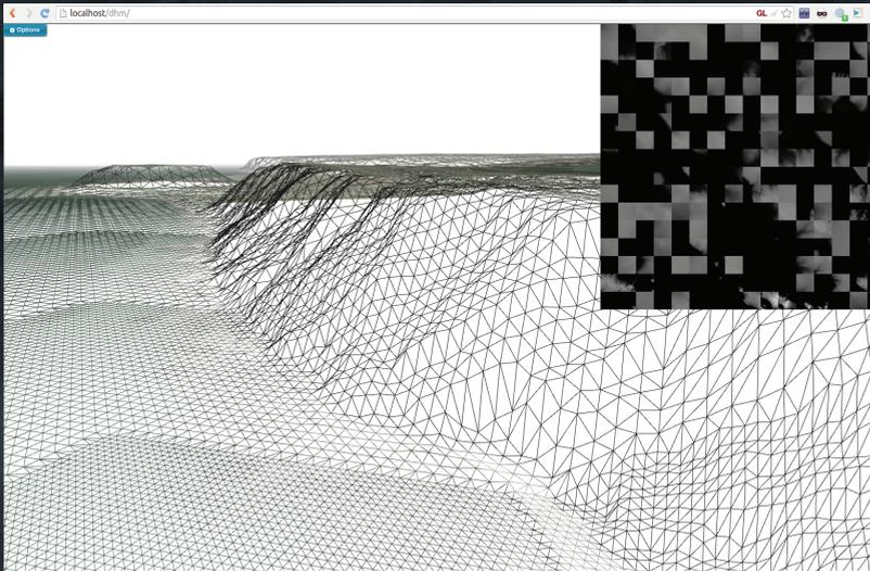
Figure 2. Caching and Level of Detail in rendering. The upper right corner shows the height map tiles that are streamed into the graphics card memory.
