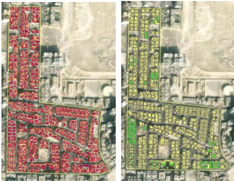
Figure 1: (a) Solar image for the site location. The selected rooftops (in green) based on the geospatial and environmental criteria.
