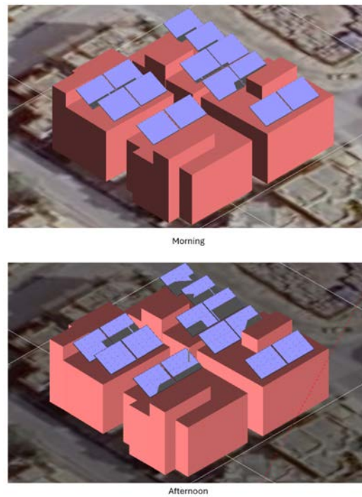
Figure 6: Shading effect on some of the selected rooftops in PVsyst.
