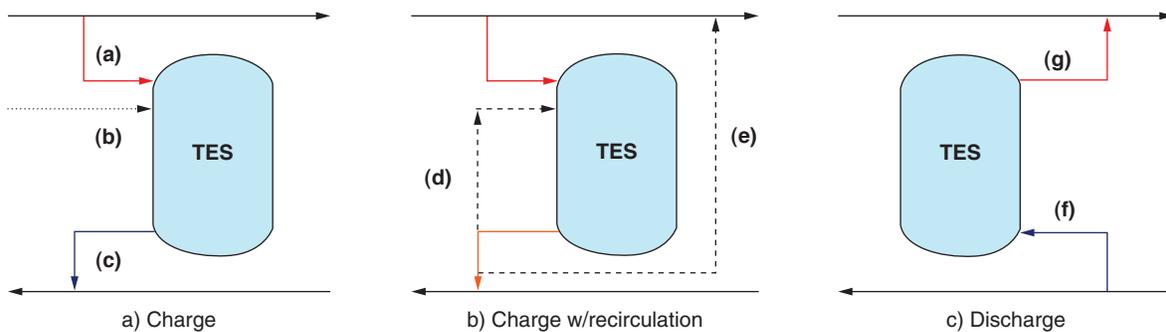
Figure 3: LH-TES system operating modes of the proposed arrangement
