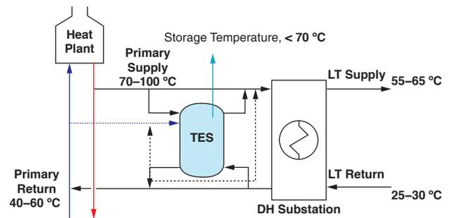
Figure 2: LH-TES system application with LTDH substation
