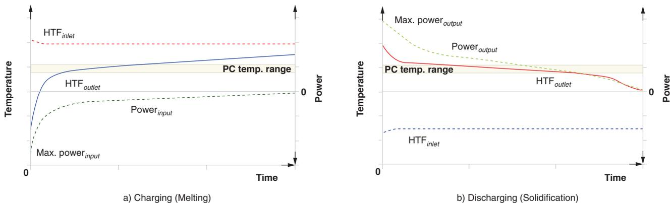
Figure 1: Characteristic temperature and power performance of active LH-TES systems
