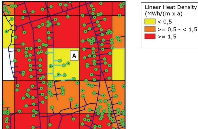
Figure 5: Analysing the linear heat density (unscaled)
