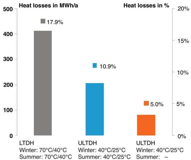
Figure 7: Heat distribution losses of the ULTDH and the LTDH network (with standard insulation)
