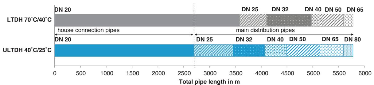
Figure 3: Nominal pipe diameter distribution showing the sum of supply and return pipes
