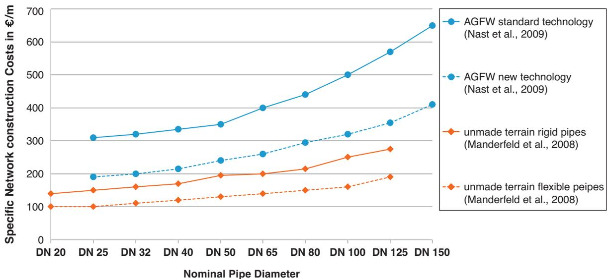
Figure 4: Specific network construction costs including construction costs and pipe material costs
