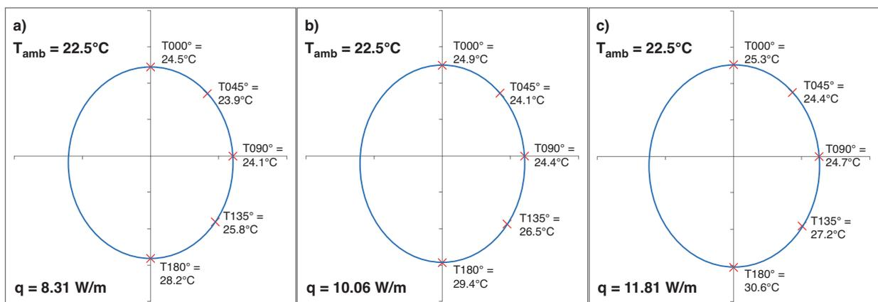
Figure 7: Temperature in the climate chamber  $T_{amb}$ ; Temperature distribution  $T(\varphi; r = R)$  on the casing and heat losses  $q$  of the PTPS for different supply flow temperatures  $T_{sup}$  a)  $T_{sup} = 70.8$  °C; b)  $T_{sup} = 79.9$  °C c)  $T_{sup} = 90.7$  °C (numerical results).
