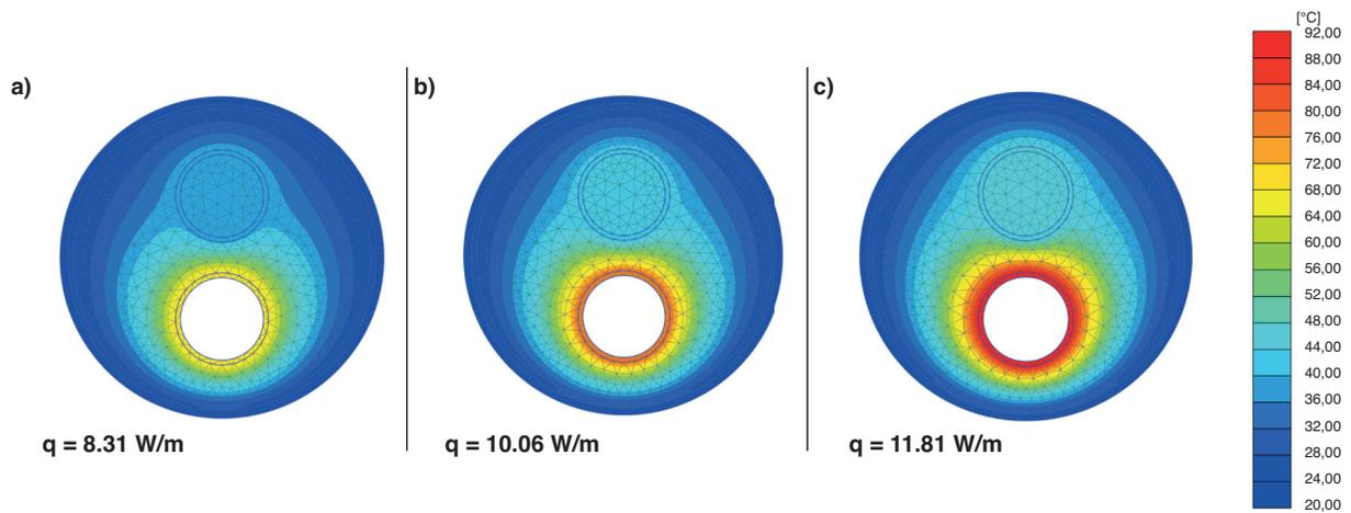
Figure 6: Temperature field  $T(\varphi; r)$  in the PTPS and heat losses  $q$  according to FEM simulations for different temperatures in the supply  $T_{sup}$  (lower pipe) a)  $T_{sup} = 70$  °C; b)  $T_{sup} = 80$  °C;  $T_{sup} = 90$  °C ( $T_{amb} = 22.5$  °C).
