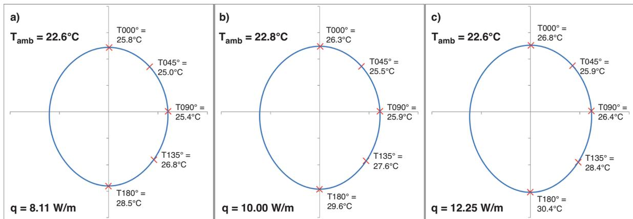
Figure 4: Temperature in the climate chamber  $T_{amb}$ ; Temperature distribution  $T(\varphi; r = R)$  on the casing and heat losses  $q$  of the PTPS for different supply flow temperatures  $T_{Sup}$  a)  $T_{Sup} = 70.8 \text{ }^\circ\text{C}$ ; b)  $T_{Sup} = 79.9 \text{ }^\circ\text{C}$  c)  $T_{Sup} = 90.7 \text{ }^\circ\text{C}$  (metrological results).
