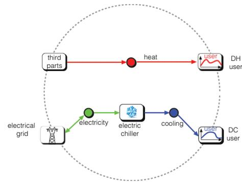
Figure 2: Present configuration of the generation units
