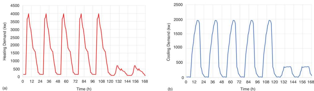
Figure 4: Aggregated weekly load profiles of the area for: a) space heating and DHW in January, b) space cooling in July
