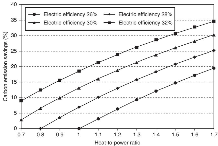
Figure 4: Carbon emission savings versus heat-to-power ratio.
