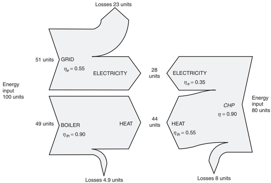
Figure 1: Schematic representation of conventional power production versus *CHP*.
