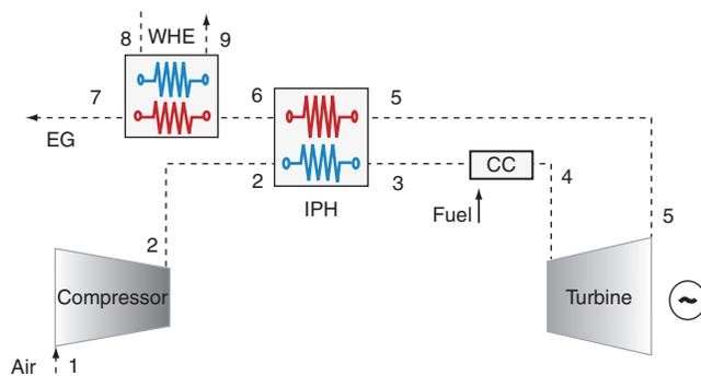
Figure 2: Schematic representation of the micro gas turbine *CHP* system.
