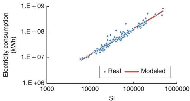
Figure 9: Comparison between the regressed and real values of residential electricity consumption in 2009.
