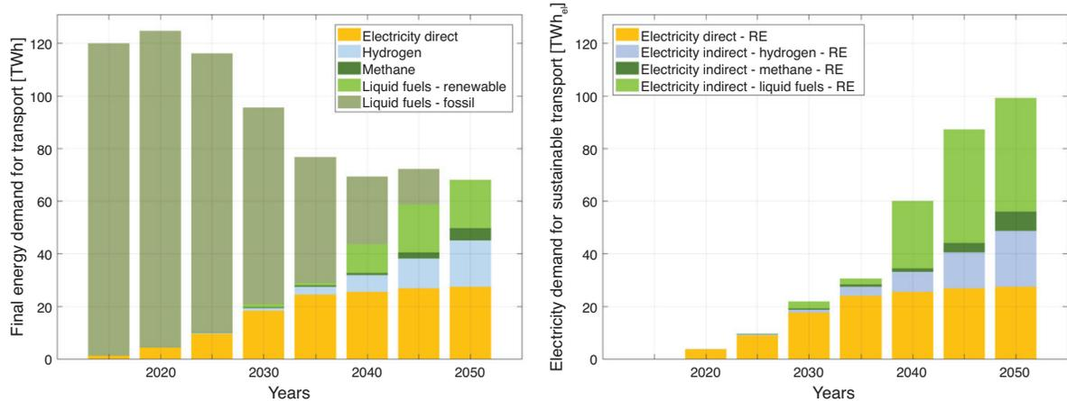
Figure 10: Final transport energy demand by fuel form (left) and electricity demand for sustainable transport (right)
