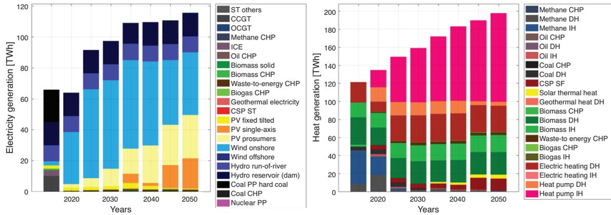
Figure 7: Power and heat - Electricity generation by power technology (left) and heat generation by heat technology (right)
