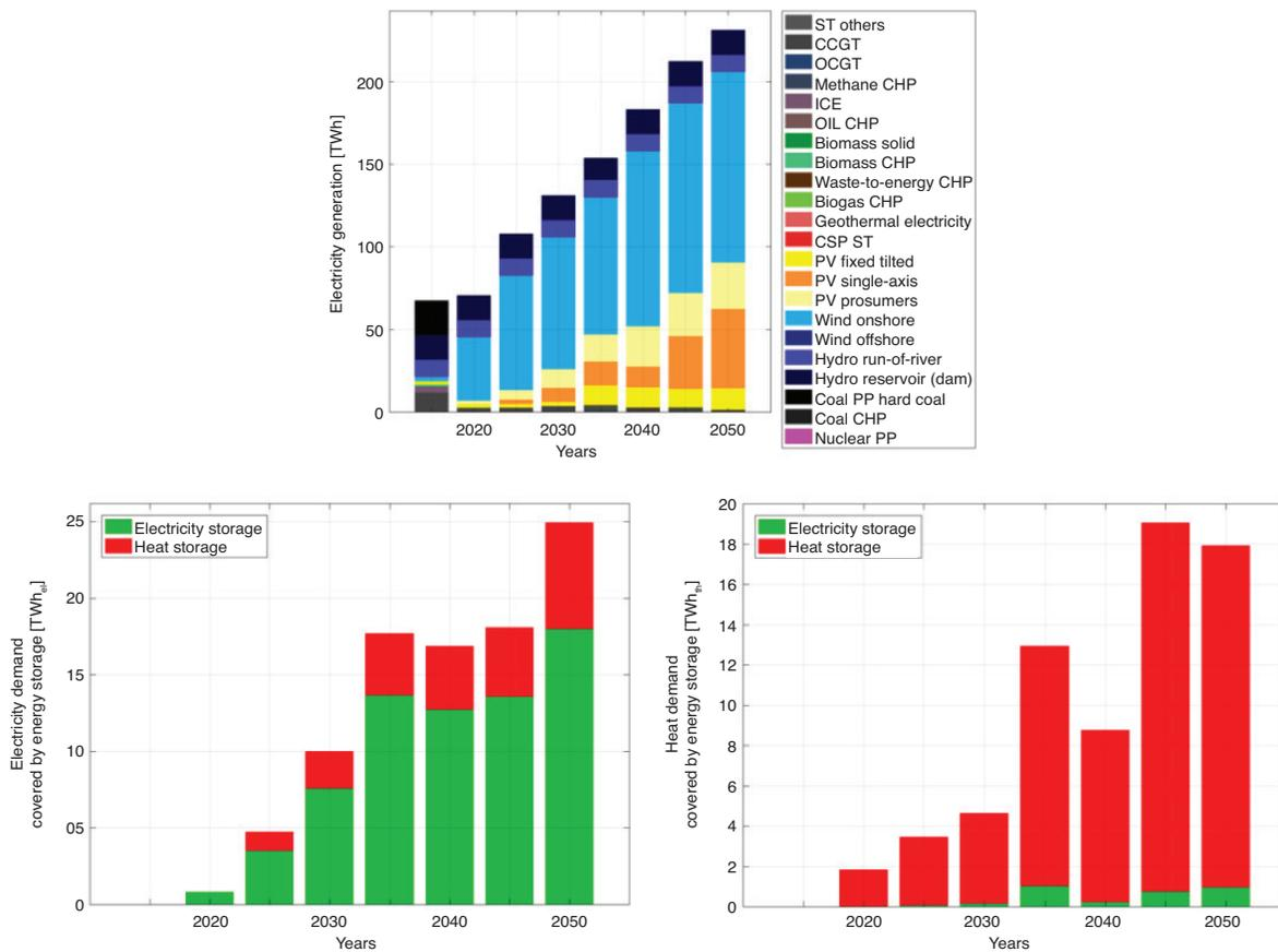
Figure 5: Technology-wise electricity generation (top), electricity demand covered by energy storage (bottom left), and heat demand covered by energy storage (bottom right) during the energy transition from 2015 to 2050
