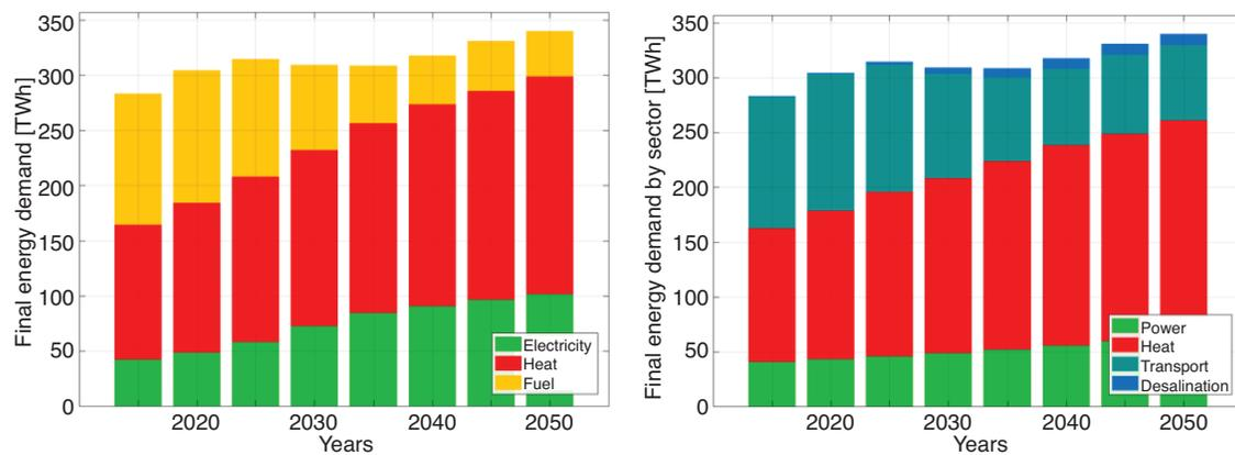
Figure 3: Final energy demand by energy form (left) and by sector (right) during the energy transition from 2015 to 2050
