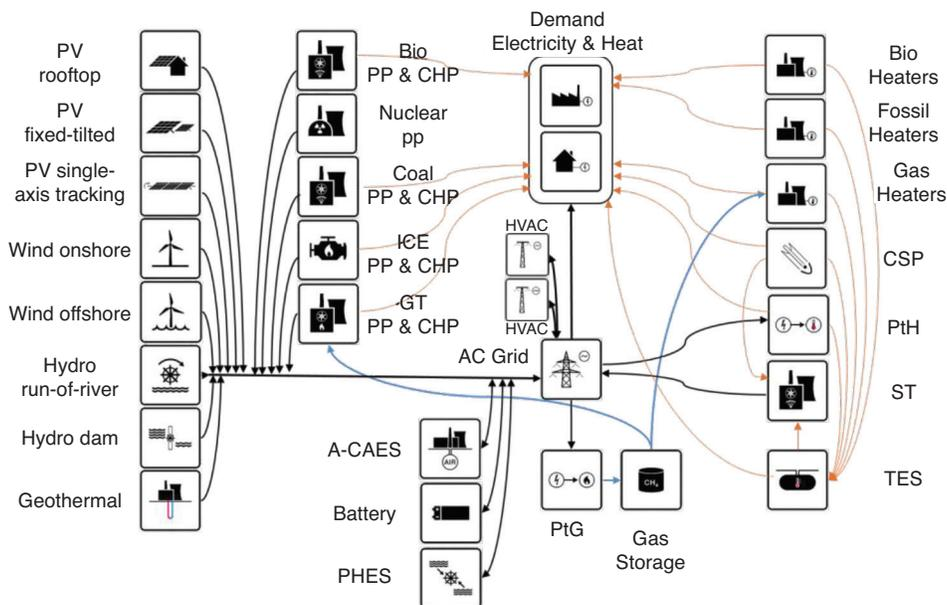
Figure 2: Schematic of the LUT Energy System Transition model for power and heat sectors [18]
