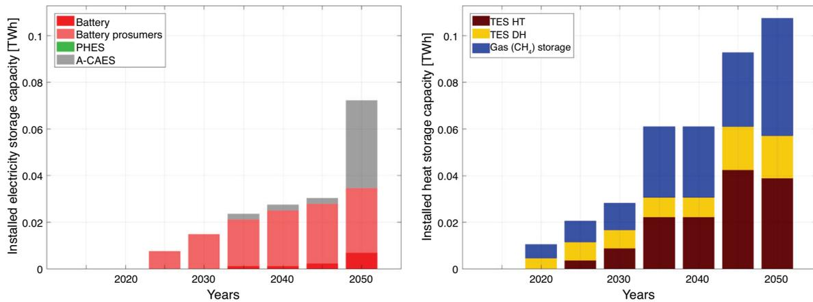
Figure 8: Power and heat - Installed electricity storage capacities (left) and heat storage capacities (right)
