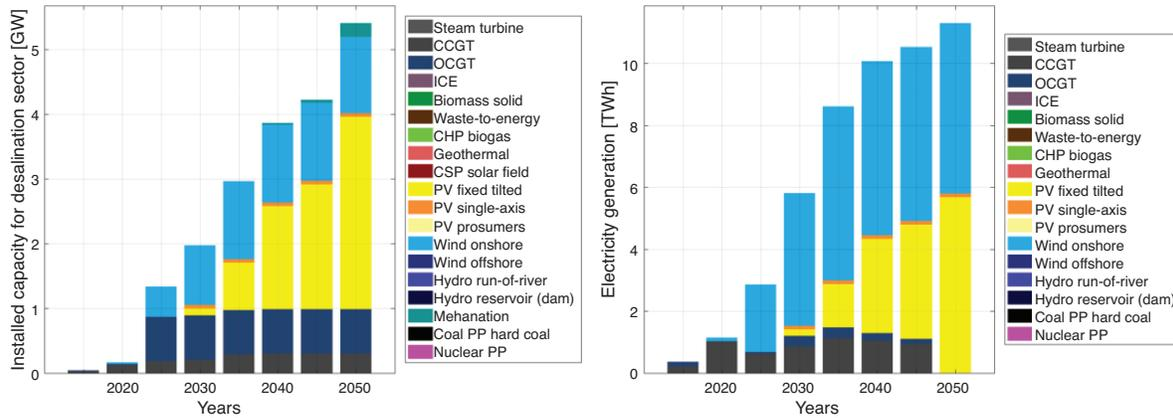
Figure 13: Desalination - Installed capacity by power technology (left) and electricity generation by power technology (right)
