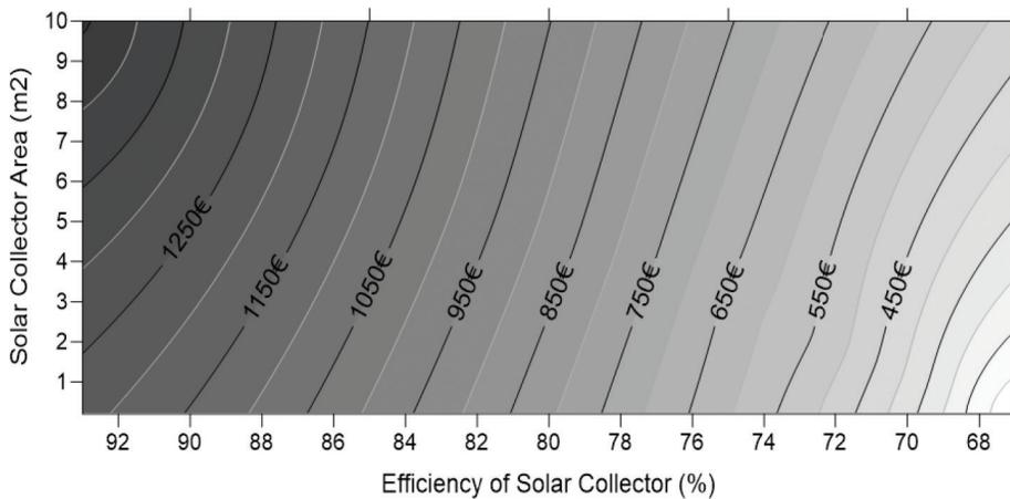
Figure 7: Cost estimation of the solar collector as a function of the collector area and its efficiency
