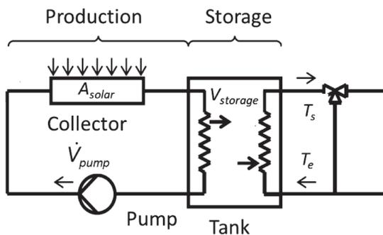
Figure 4: Scheme of the main circuit of the solar thermal system
