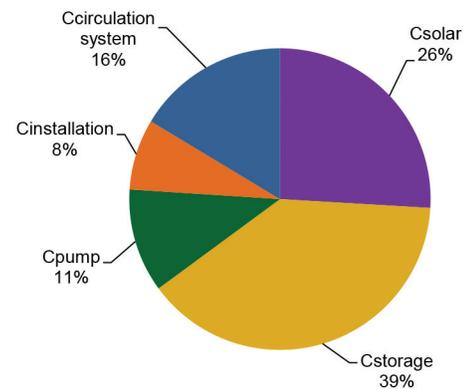
Figure 9: Breakdown of the investment costs (storage tank of 0.36 m<sup>3</sup>)
