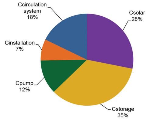
Figure 8: Breakdown of the investment costs (storage tank of 0.24 m<sup>3</sup>)
