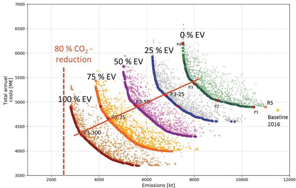
Figure 9: Pareto fronts evaluated for different penetrations of EV, Baseline 2016, Reference Scenario, scenarios from P1 to P4 on the 0% EV Pareto front. Scenarios from P3-25 to P3-100 chosen at the same point on the Pareto front of P3
