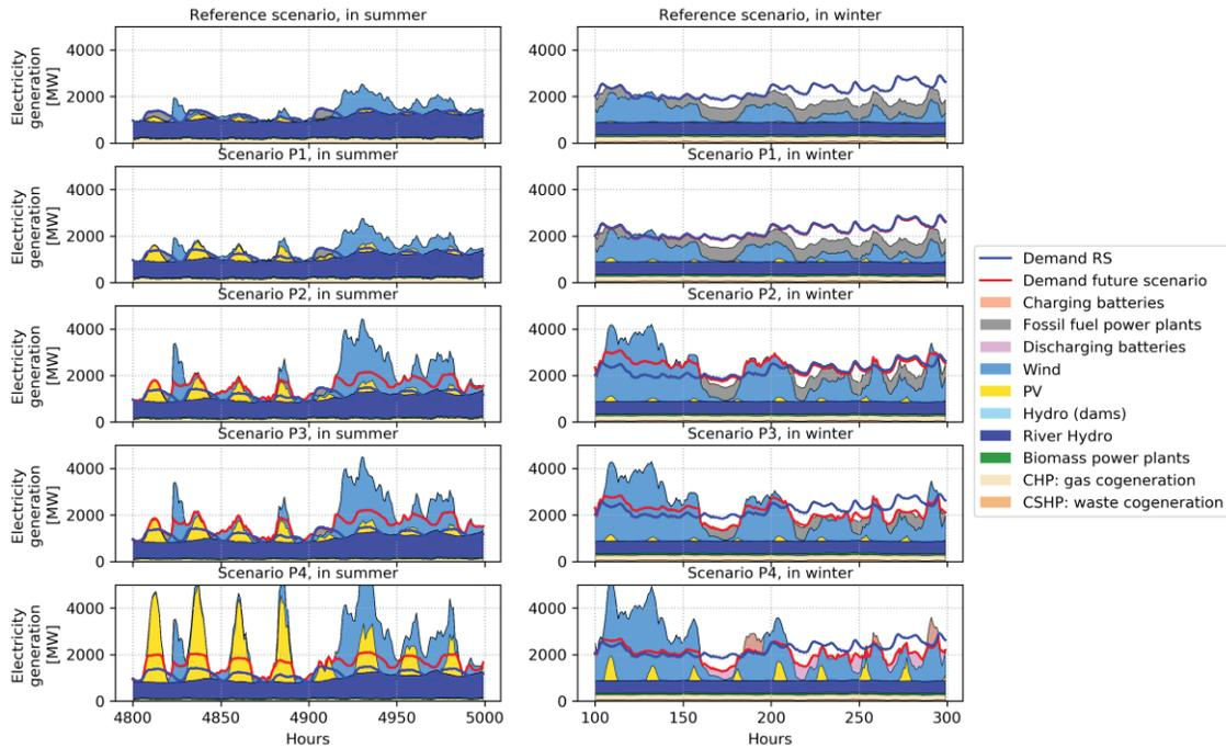
Figure 6: Hourly electricity dispatch for two weeks of the year (one in summer and one in winter) for the scenarios RS, P1, P2, P3 and P4
