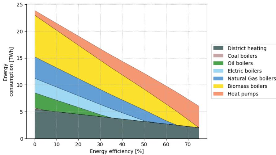
Figure 3: Theoretical decrease of final energy consumption due to energy efficiency
