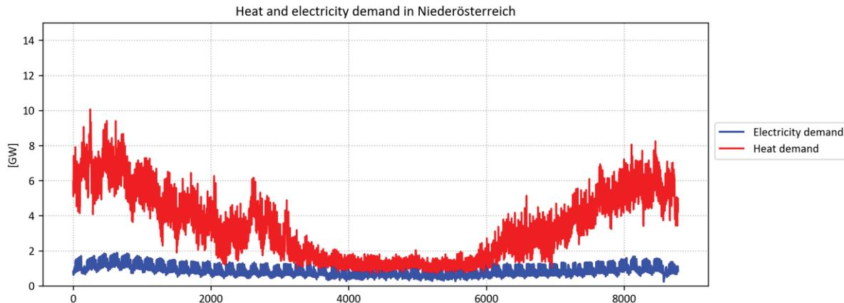
Figure 2: Comparison between the heat and electricity demand during the year
