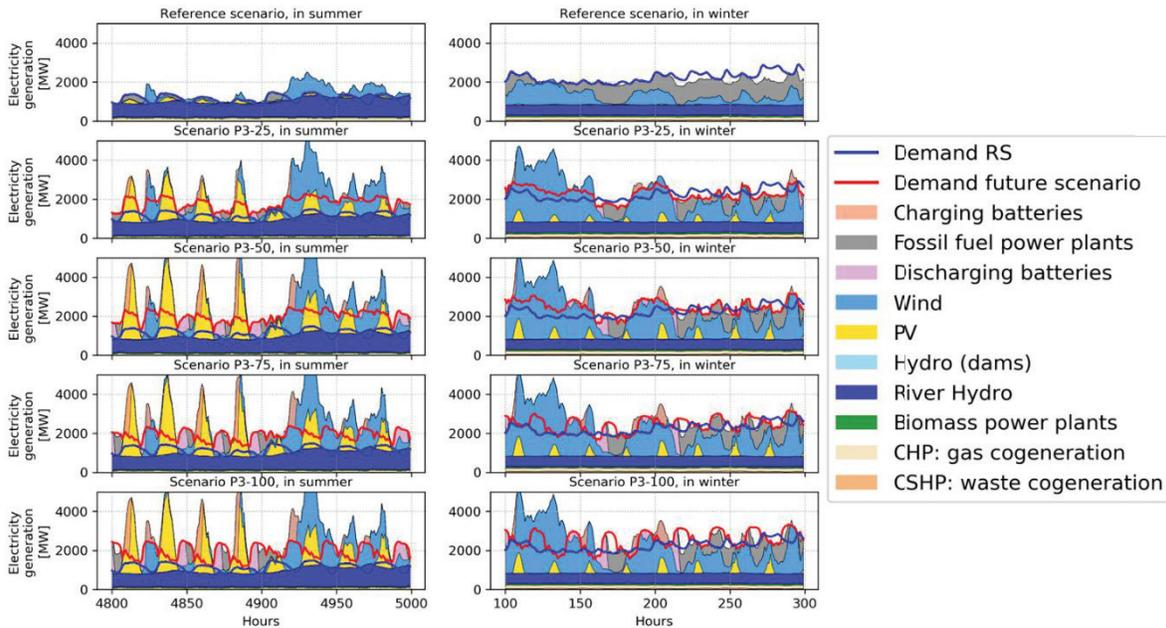
Figure 11: Hourly electricity dispatch for two weeks of the year (one in summer and one in winter) for the scenarios RS, P3-25, P3-50, P3-75 and P3-100
