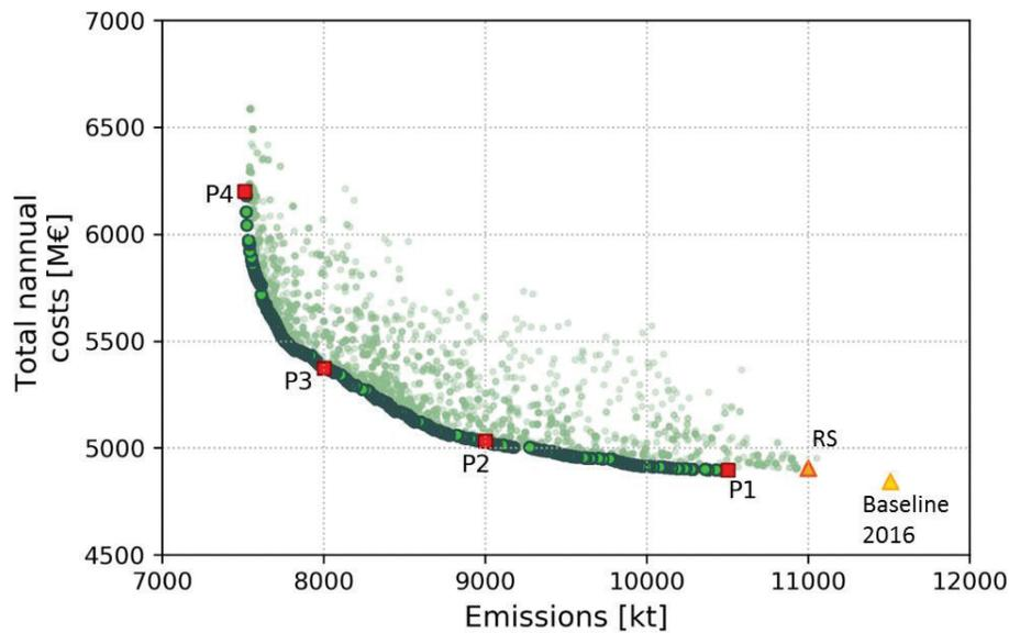
Figure 4: Evaluated scenarios: Baseline 2016, Reference Scenario, clouds of dominated solutions and Pareto front of optimal solutions. Four scenarios are selected to inspect the results on the Pareto front: P1, P2, P3 and P4
