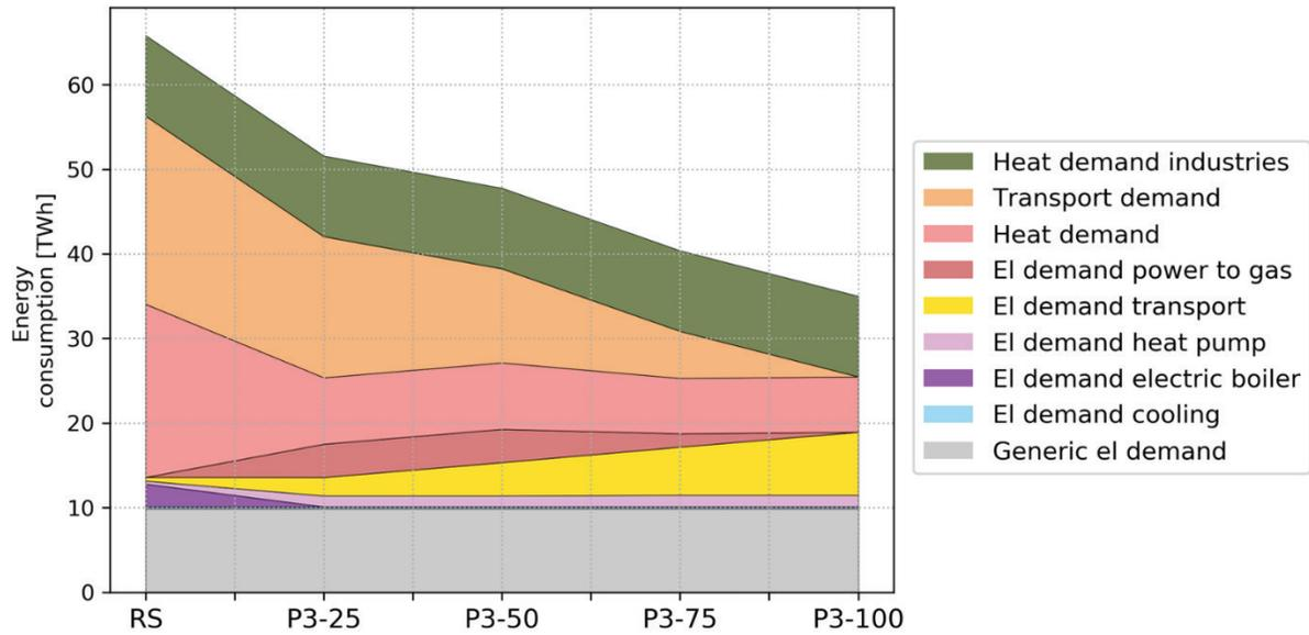
Figure 12: Energy consumption in the four main sectors of the energy system: electricity, heat, industry and transport for the scenarios RS, P3-25, P3-50, P3-75 and P3-100
