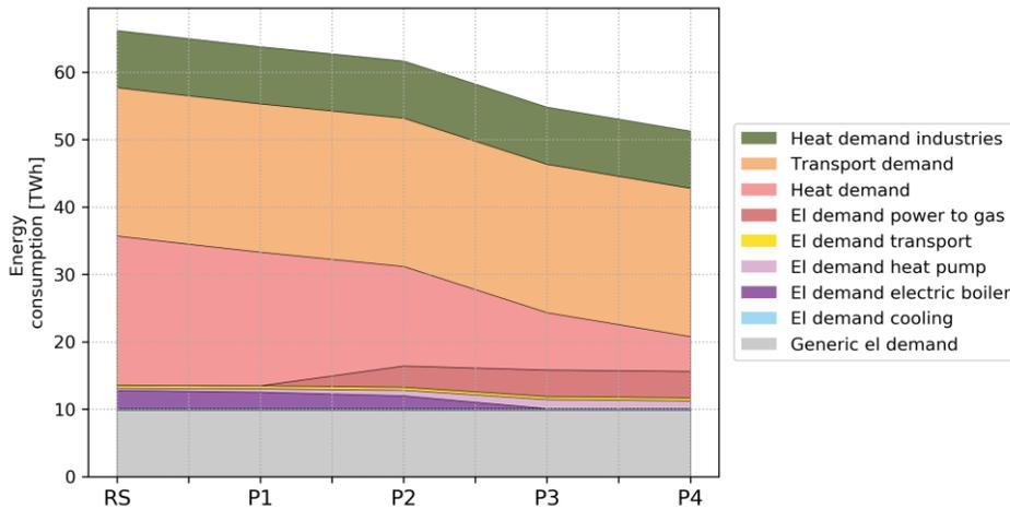
Figure 7: Energy consumption in the four main sectors of the energy system: electricity, heat, industry and transport for the scenarios RS, P1, P2, P3 and P4
