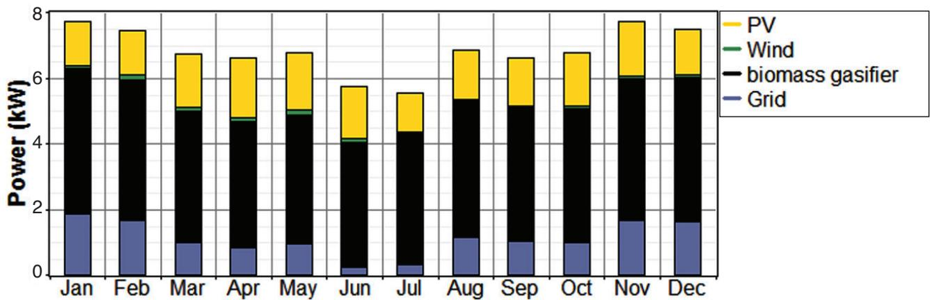
Figure 9: Monthly average electricity production of generation units in Case 2
