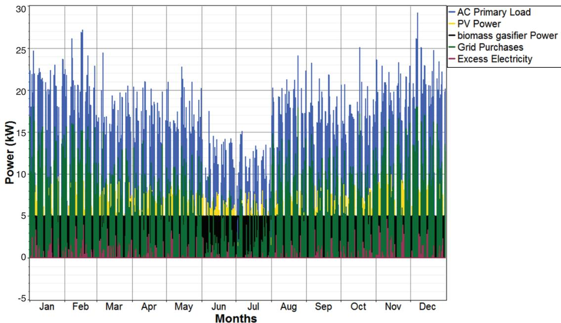
Figure 13: Hourly electricity generation from PV/Biomass/Grid hybrid system
