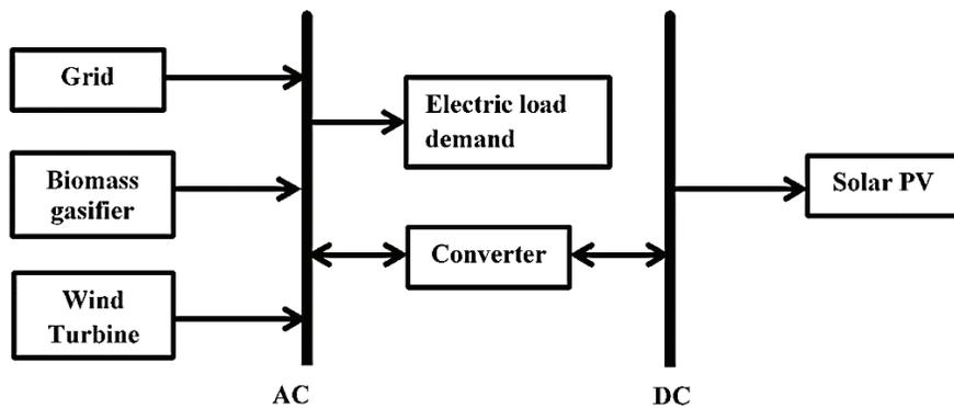
Figure 8: On-grid hybrid energy system for Case 2
