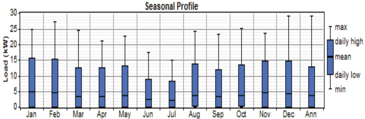
Figure 4: Month-wise electric load profile of CEEE building
