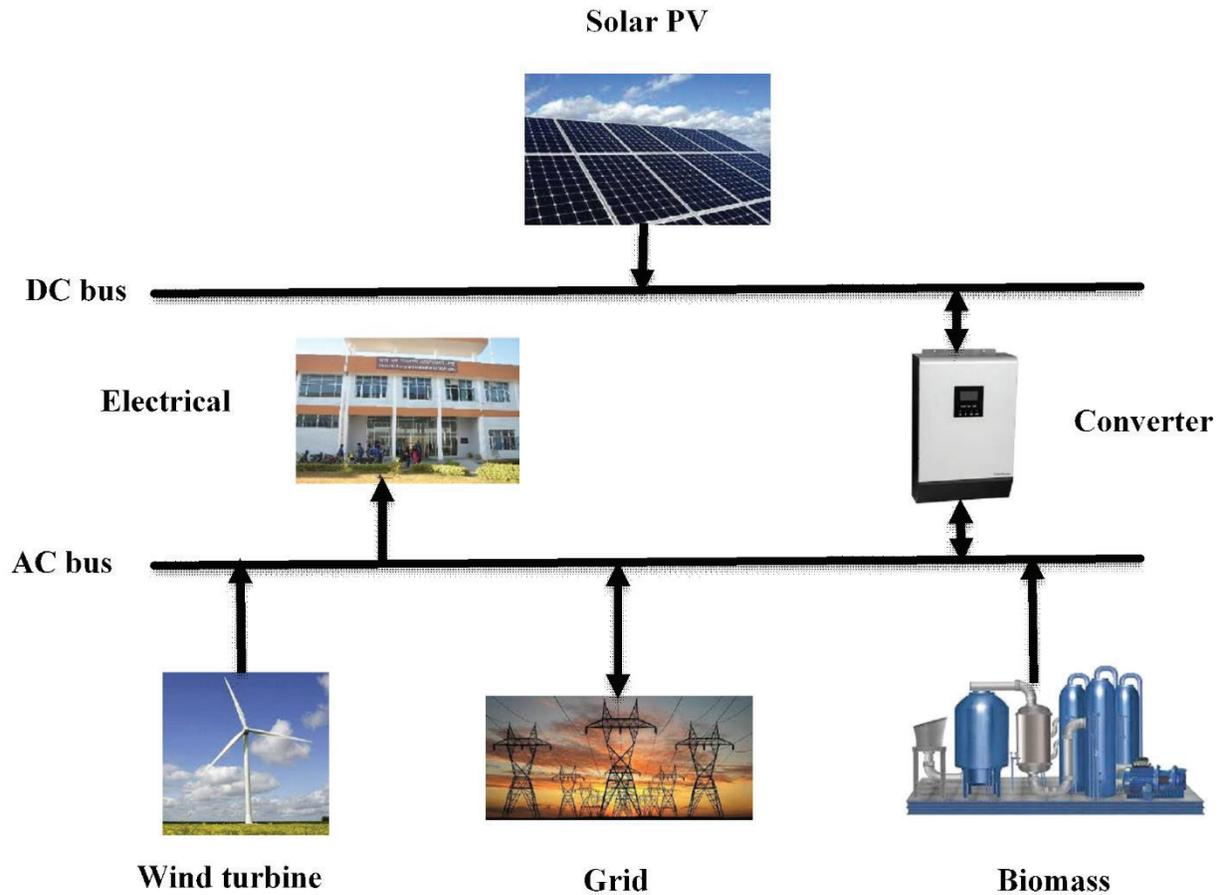
Figure 5: The schematic diagram of the proposed hybrid energy system
