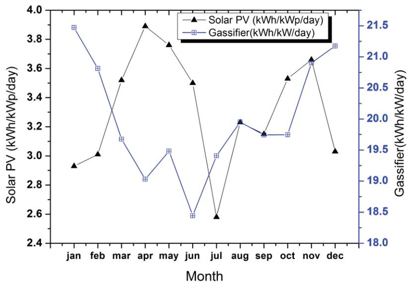
Figure 15: Power generation from PV and Biomass system
