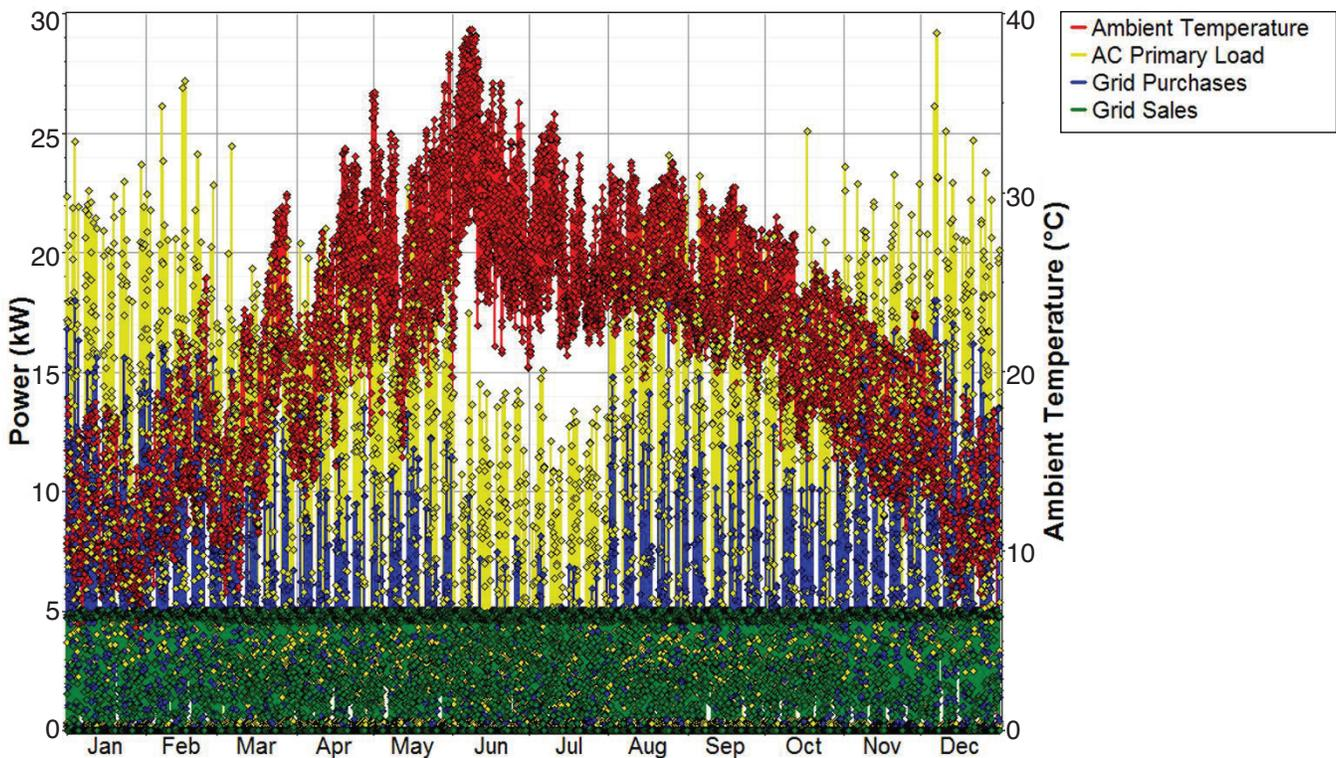
Fig. 14: Monthwise hourly grid import and export power along with load demand and ambient temperature
