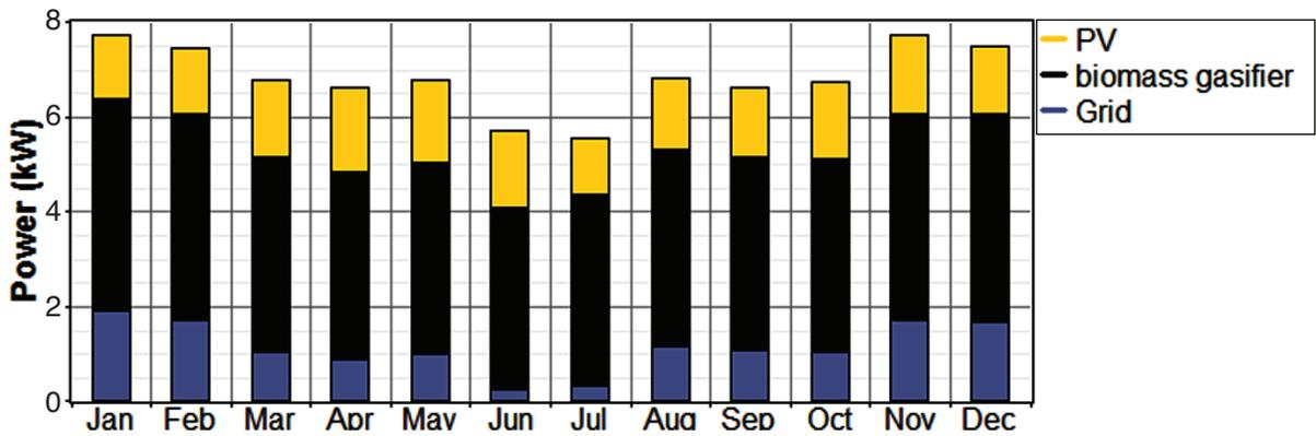
Figure 7: Monthly average electricity production of generation units in Case 1
