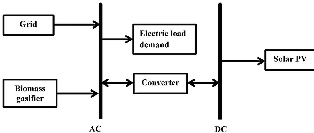
Figure 6: On-grid hybrid energy system for Case 1
