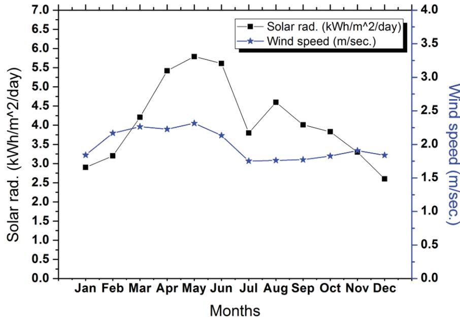
Figure 3: Monthly average global solar radiation and wind speed at CEEE, Hamirpur (H.P.)
