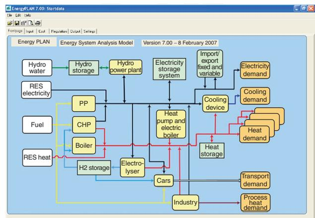
Figure 1: Overall structure of the EnergyPLAN model. Screenshot from the model.
