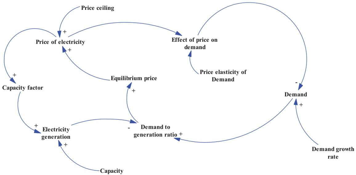
Figure 5: CLD of the electricity demand module
