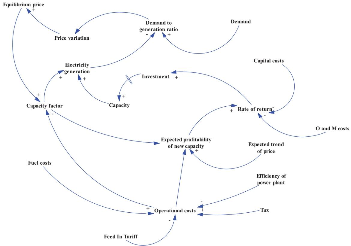
Figure 4: CLD of the electricity production module
