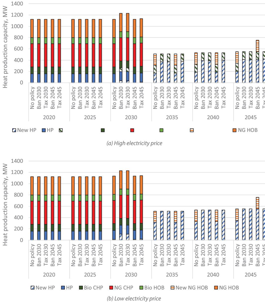
Figure 5 Capacity of DH supply plants. EH and MSW incineration remain unchanged and have been left out in the figures to improve readability. Also, oil HOB and electric HOB available from the starting year but are never utilized are left out to improve readability.
