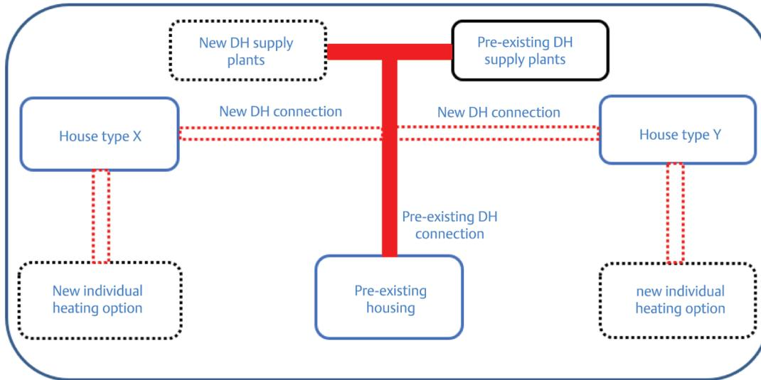
Figure 2. Schematic representation of the model setup for determining the cost optimal heating solution with different types of new housing.
