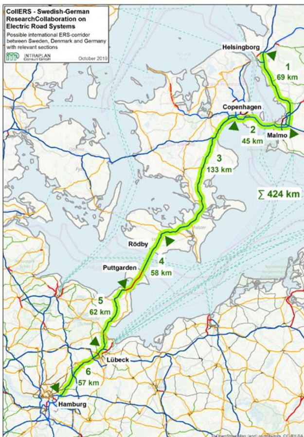
Figure 1: Chosen corridor route for the feasibility study
