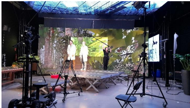
Figure 1: BUAS XR stage: digital camera with motion capture (MoCap) 4 crown on a cart (left), stage area with actors on adjustable platforms, boom operator and LED volume in the background (middle), upper LED volume (top), traditional light projector on a tripod, and led light panel (right). Training session photograph by the VPSN team in 2024.
